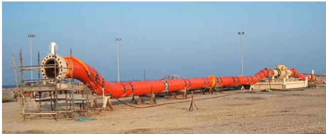
Image 1 - Test spool with survey control targets (52 meters between the end targets)
